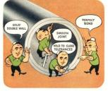
4. BUNDYWELD is different from other tubing. A single strip of basic metal, coated with a bonding metal rolled continuously twice laterally into tubular form, then metallurgically bonded by intense heat—carefully control of the form a solid, double wall tube, held to close dimensions.
