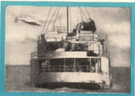
Automatically following every change in course of enemy ship—the Bat hits the target. First such weapon successfully used in combat by any nation. (*Sponsored by U. S. Navy Bureau of Ordnance and Bureau of Standards, the Bat is 12 feet long, has a 10-foot wing span. Official U. S. Navy photographs.)
