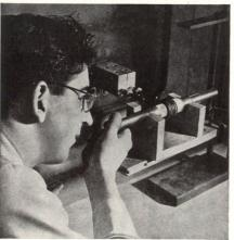
Today, an ingenious production tool the Electronic Heater, developed by Allis-Chalmers—applies Industry's new Induction Heating principles to the heat-treating of many different kinds of metals. By producing a rapidly alternating magnetic field around a simple copper work coil (see cut above), the Electronic Heater makes metals "cook" in their own heat . . . greatly simplifies dozens of hardening, soldering, brazing and annealing operations in industry.
