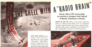
by the target, the returning wave explodes the shell automatically and at the correct instant.
