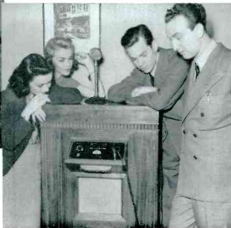
THE "STEEL TAPE" MACHINE (Right) plays back the tune for the youngsters to hear their mistakes, if any, and then allow for final corrections. The excellent part of this process is the fact that this recording keeps repeating itself without any winding or changing of needles. The tune plays over and over until the switch is thrown.
