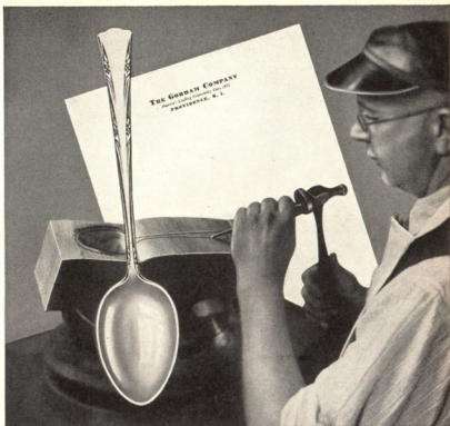
Gorham master craftsman cutting the die for GREENBRIER, newest Sterling pattern
