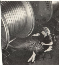
④ Each of the three thousand, six hundred thirty-six wires in this cable is given a thorough electrical test.
